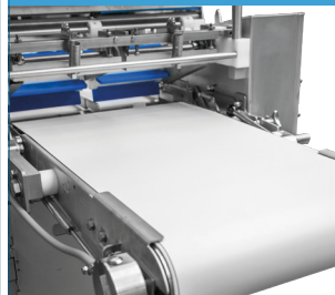
Short outfeed conveyor = -549mm
